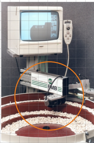
Location examination of ceramic parts integrated into a sorter.
