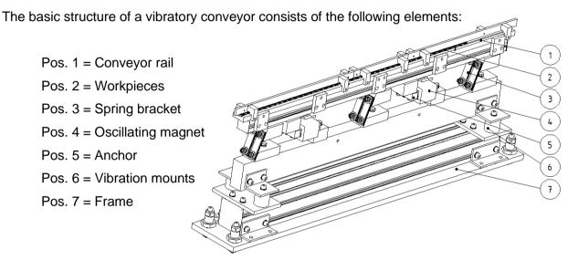
If the magnet that is permanently connected to the counterweight, electricity is supplied, it produces a force that attracts the armature, depending on the resonant frequency of the network and releases.
