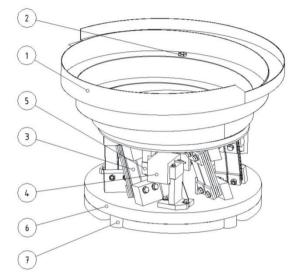
If the magnet that is permanently connected to the counterweight, electricity is supplied, it produces a force that attracts the armature, depending on the resonant frequency of the network and releases.
