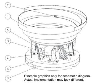
If the magnet that is permanently connected to the counterweight, electricity is supplied, it produces a force that attracts the armature, depending on the resonant frequency of the network and releases.
